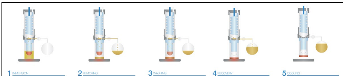
Figure 1: Extraction process with the VELP SER 158 Automatic Solvent Extractor, which includes immersion, removing, washing, recovery, and cooling steps (acquired picture from 14)
