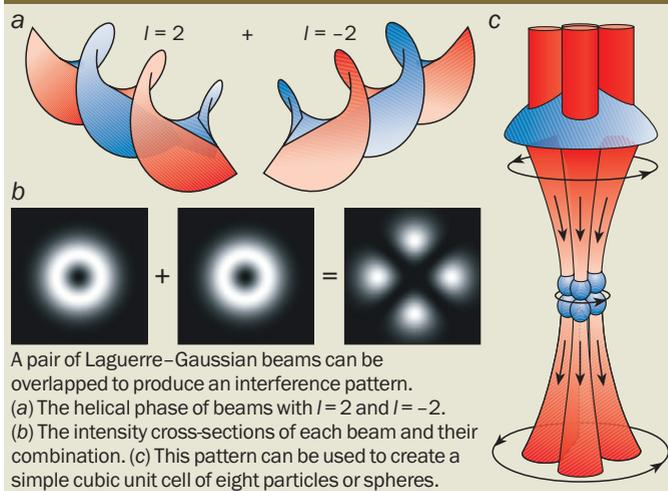
possible to grab and move dielectric objects and biological samples – ranging in size from tens of nanometres right up to tens of microns – at will. Although the optical forces might only be of the order of piconewtons, such forces can often be dominant at the micro-level.
